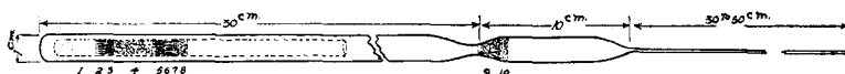
Fig. 2.—(1) Magnesite. (2) Asbestos. (3) Lead chromate. (4) Dried precipitate ground with lead chromate. (5) Lead chromate. (6) Asbestos. (7) Sodium carbonate. (8) Glass wool. (9) Glass wool. (10) Phosphorus pentoxide.
